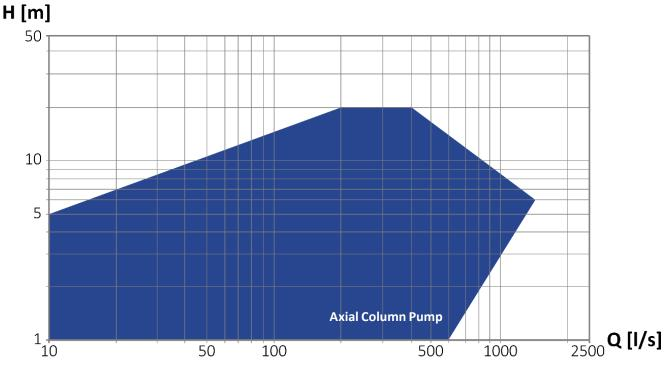
Range chart for the entire product group Axial Column Pumps. Pumps with higher flow rates up to 10'000 l/s are available from Bedford Pumps.
